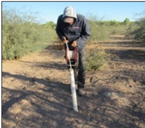
Figure 51. Measuring groundwater levels in the CILA restoration site
