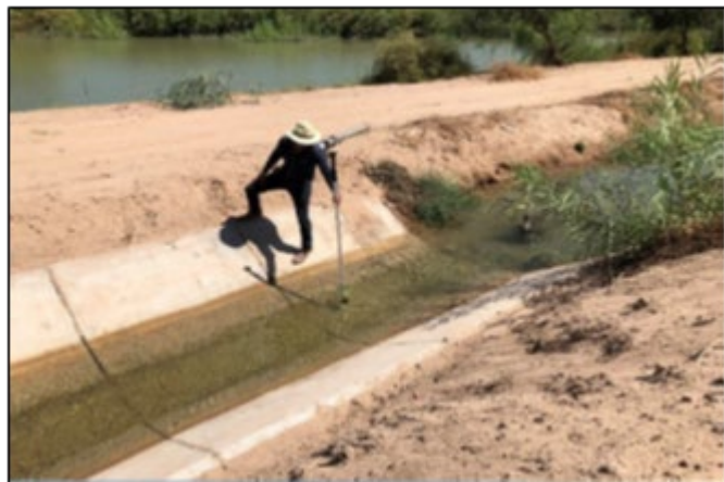
Figure 52. Measuring flows in a canal in the Herradura restoration site.
