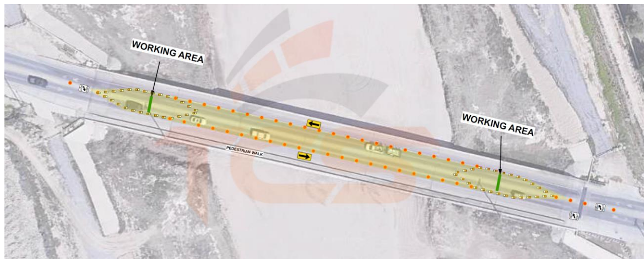
Phase 4: Traffic Lanes Separated (Westbound Lane Shifts to North Shoulder)
