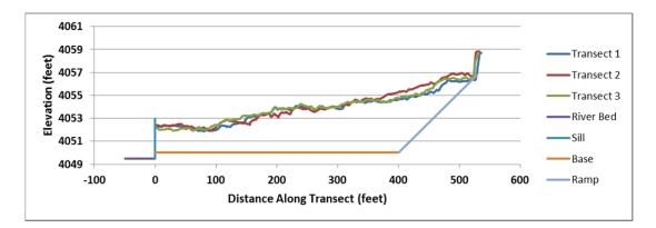
Figure A-17. Cross-Section of Basin-Based Trap and Geometric Parameters (Sill, Base, Ramp)
