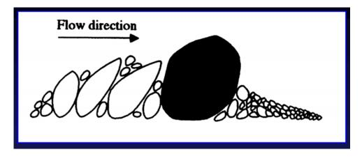
Figure A-16. Schematic Showing Hiding and Exposure of Variable-Sized Grains
