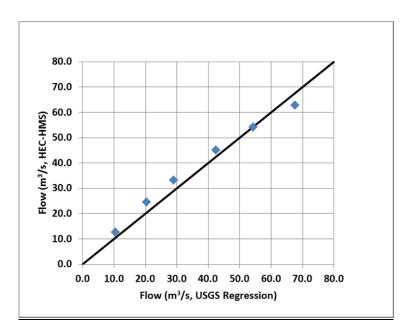
Figure A-9. Comparison of USGS Regression-Based Discharges and Results of Return Period Analysis of Model Output for Thurman II Arroyo
