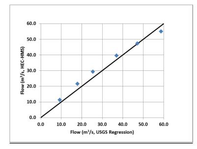
Figure A-8. Comparison of USGS Regression-Based Discharges and Results of Return Period Analysis of Model Output for Thurman I Arroyo
