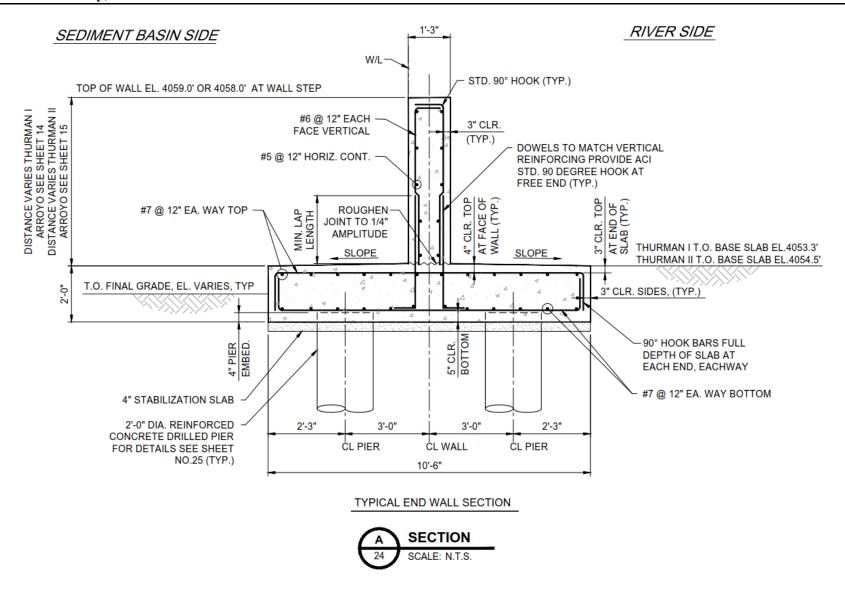
Figure 7-1. Proposed Pier-Supported Floodwall
