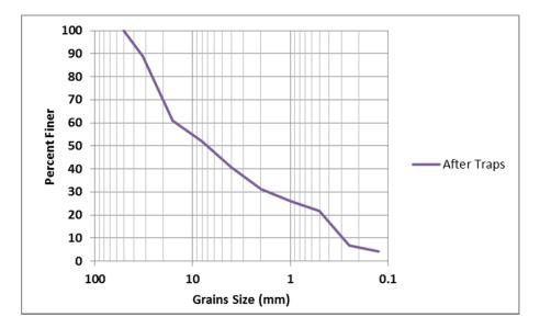
Figure A-14. Grain Size Curve of Sediment Estimated to Pass Through the Mesh-Based Trap
