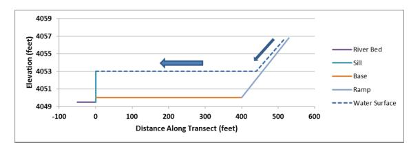
Figure A-19. Water Elevation and Flow Paths in Basin
