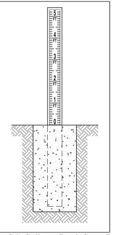
Figure C-2. Sediment Depth Gauge Detail
