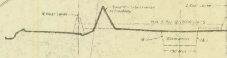
CROSS SECTION A-A Hor Scale=1"=100' Vert Scale=1"=40'
