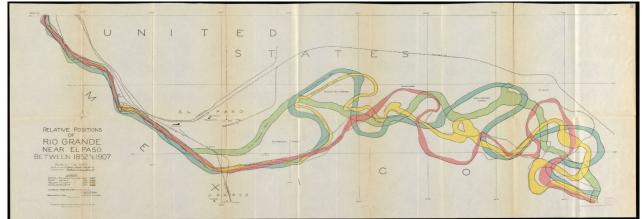
Pictured: Relative positions of the Rio Grande near El Paso between 1852 and 1907 showing how the river meandered before the channelization. Map provided by USIBWC Records Management Division
