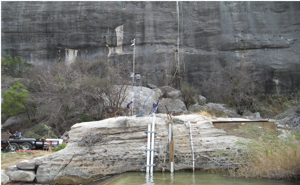
Pictured: Setup of the CWQM station at Langtry by staff with the USGS.
