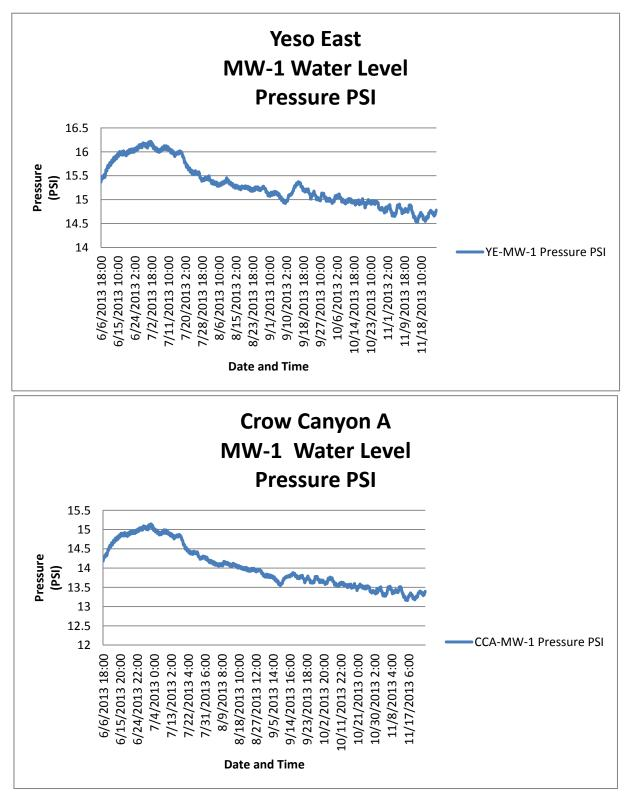
Note: Due to dry conditions, the transducer for Crow Canyon B did not produce usable results.
