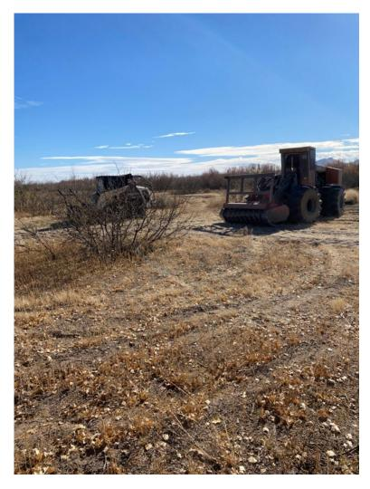
Figure B-26. Barko 937 Mulcher and Terex R350T Skid Steer with Toshhog Mulching Head (Photo #164)
